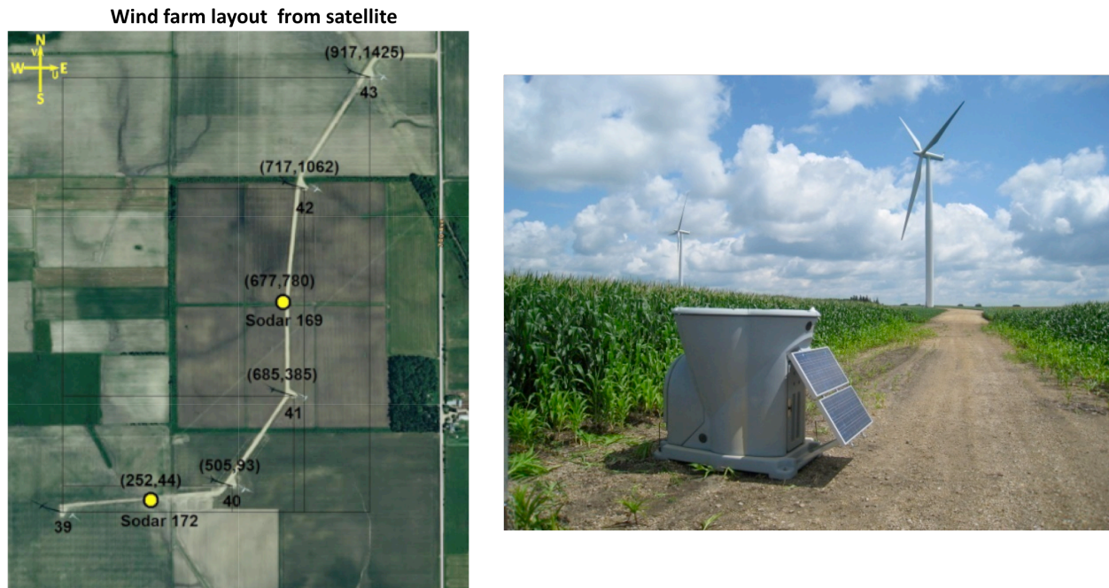
Figure 3. Left: Satellite image of the South-West corner of the Mower County Wind Farm, where the field campaign is under way. Coordinates indicate location of the turbines and SODARS (represented by yellow dots). Right: Picture of SODAR-169 and wind turbines 41 and 42 in the background.
